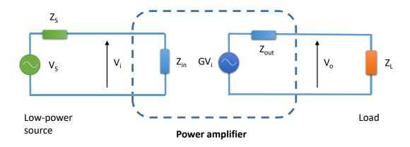
The maximum output voltage that both models of amplifier can deliver to a given load Z<sub>L</sub> are:
